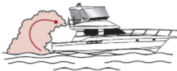
Figure 3. When protective weather coverings are in place, engine or generator exhaust from your yacht, while docked and/or running, can cause excessive accumulation of Carbon Monoxide gas within the cabin and cockpit areas of your yacht. Always provide adequate ventilation when the weather coverings are in place and either the engine or generator are running.
