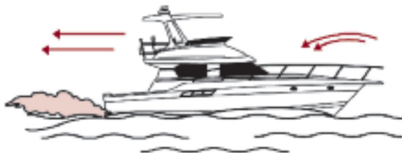
Figure 4. Engine or generator exhaust from your yacht while underway and operating with a high bow angle can cause excessive accumulation of Carbon Monoxide gas within the cabin and cockpit areas of your yacht. Always provide adequate ventilation and redistribute the load to lower the bow angle.
