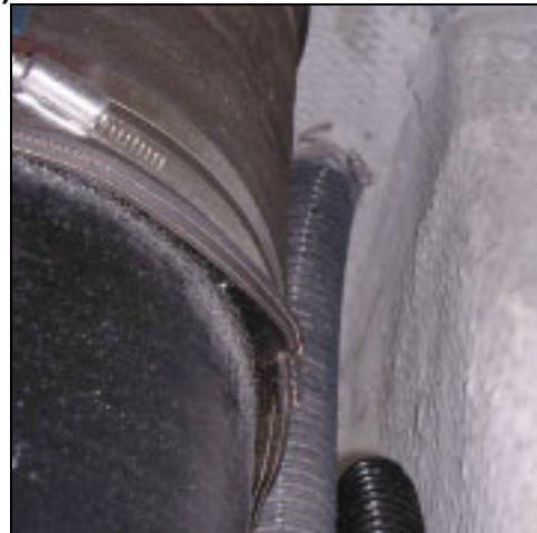
Figures 1 and 2- Central Drain Thru-Hull Location- Port Transom
